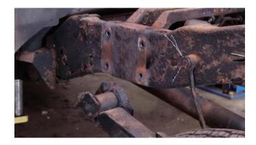
Hold the part up to the frame using the frame holes for alignment and take note of its coverage. Mark off any sections you wish to cut off, while leaving enough to weld back on to.
