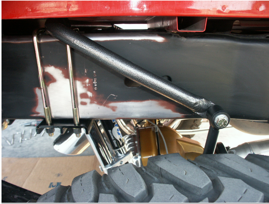
Figure 9: sway bar end link mounted to sway bar
