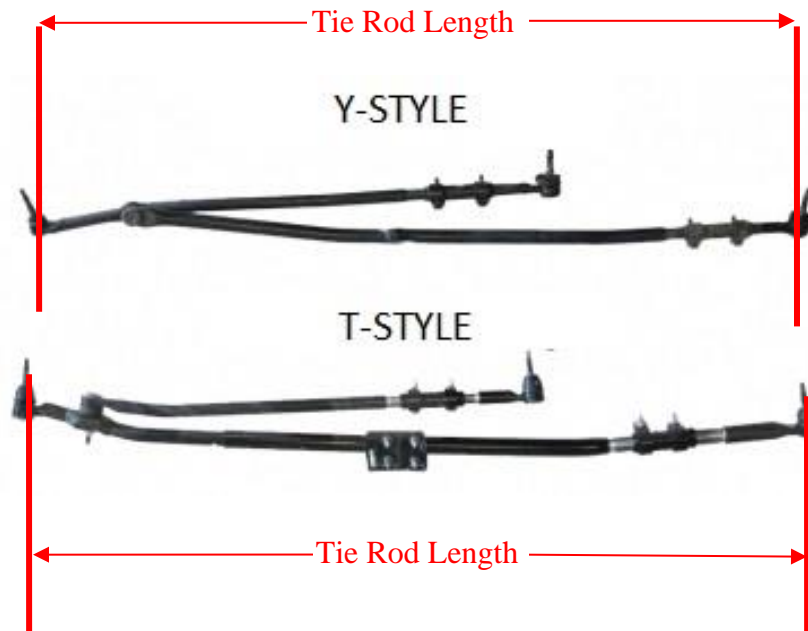
Figure 1. How to Measure Tie Rod Length
