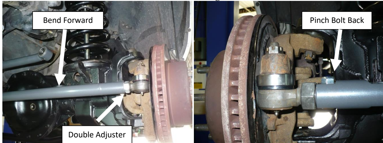
Figure 12 and 13. 2003-2013 Tie Rod Shown with Pinch Bolts Back and Bend Forward
