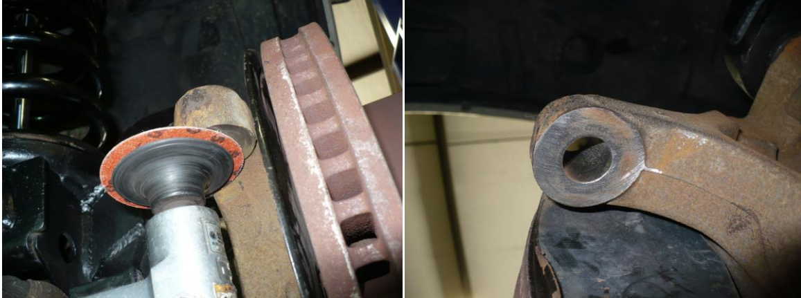
Figure 6 and 7. Smoothing Bottom of Steering Knuckle
