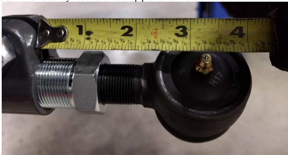
Figure 23. Tie Rod End Adjusted MAX 3.25" Out (Double Adjuster Side)
