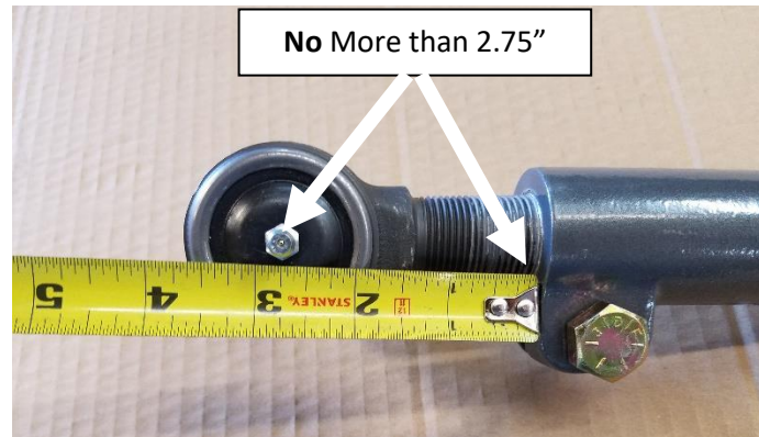
Figure 20. Tie Rod End Adjusted MAX 2.75" Out (Non Double Adjuster Side)
