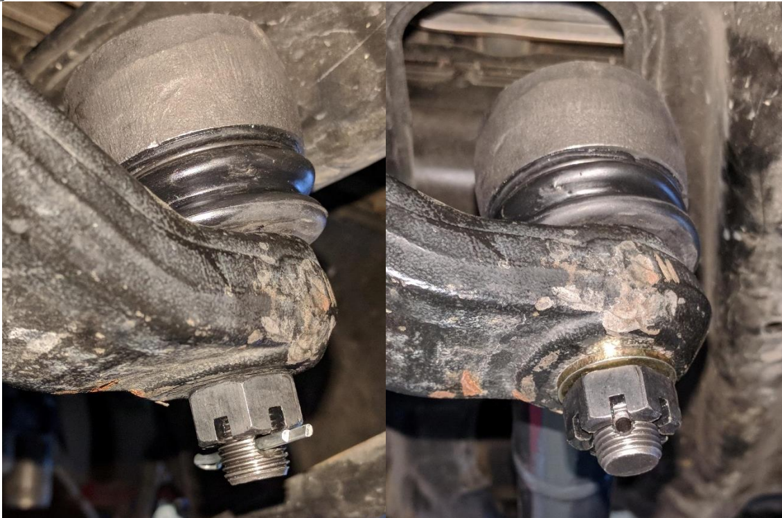
Figure 24 and 25. Washer Used Under Castle Nut
