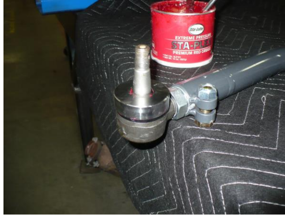
Figure 5. Bushing and Cap Installed
