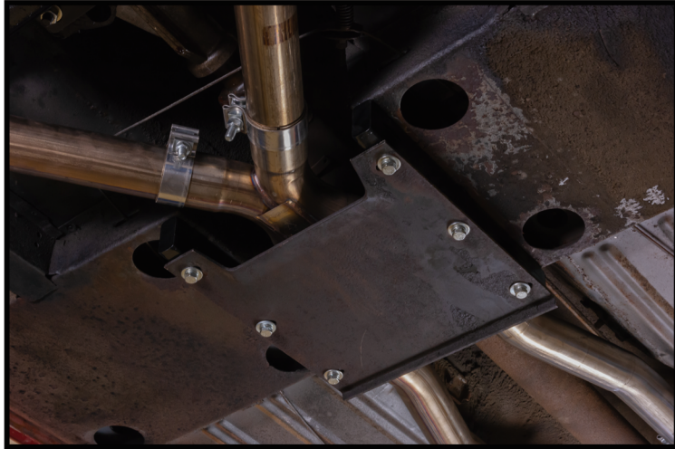
SHOWN ABOVE BRACE SPACER KIT INSTALLED
