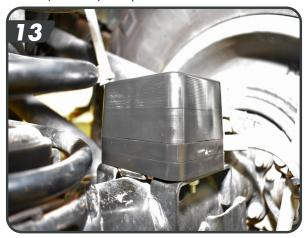
v. The shocks come with the bushings and upper spacers pre-installed. The wide mount will be installed up, at the frame. Slide the shock up into the mount. The longer shocks will be used in the rear. JSPEC shocks will be installed body down, Fox shocks will be installed body up.
