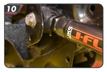
**HINT:** If mounting bolt is difficult to install due to misalignment of control arm bushing with mounting bracket, either (¹) adjust height of axle housing with hydraulic jack, or (²) move axle housing into position with a heavy-duty ratchet strap.
