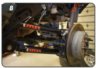
h. Mount the control arm to the frame bracket with the grease fitting up. Install the original mounting bolt and flag nut. Finger tighten the bolt. [9] DO NOT torque mounting hardware until instructed.
