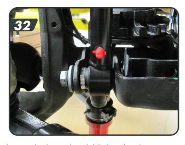
au. Install the remaning longer sleeve on the driver side and slide the polyurethane spacer onto the sleeve so it will mount towards the axle mount tab. Install the quicker disconnect to the inboard side of the axle tab with the original sway bar link hardware.
