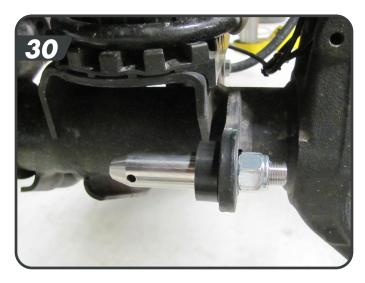
an. The kit comes with disconnect retention brackets to hold the links when the links are disconnected. Install the retention brackets using the provided 5/16" bolts into the factory hole in the front of the coil bucket [31]. These are designed to slightly interfere with the edge of the coil bucket to hold them in place.
