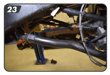
**HINT:** If mounting bolt is difficult to install due to misalignment of the control arm bushing with mounting bracket, either (¹) adjust height of axle housing with hydraulic jack, or (²) move axle housing into position with a heavy-duty ratchet strap.
