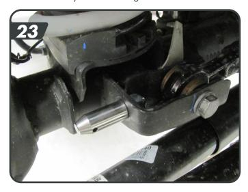
p. Install the longer disconnect post on the driver side axle sway bar link mount with it pointing inboard [24]. Fasten with the  $\frac{1}{2}$ " nylock nut and tighten to 64 ft-lbs. Tighten the post with the pin hole parallel to the ground. Slide the polyurethane spacer on the pin up against the axle tab.
