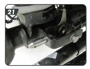
Install the longer disconnect post on the driver side axle sway bar link mount with it pointing inboard [22]. Fasten with the ½" nylock nut and tighten to 64 ft-lbs. Tighten the post with the pin hole parallel to the ground. Slide the polyurethane spacer on the pin up against the axle tab.
